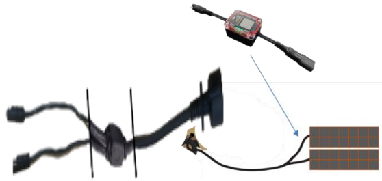
Figure 1-3. Power Meter Connection
